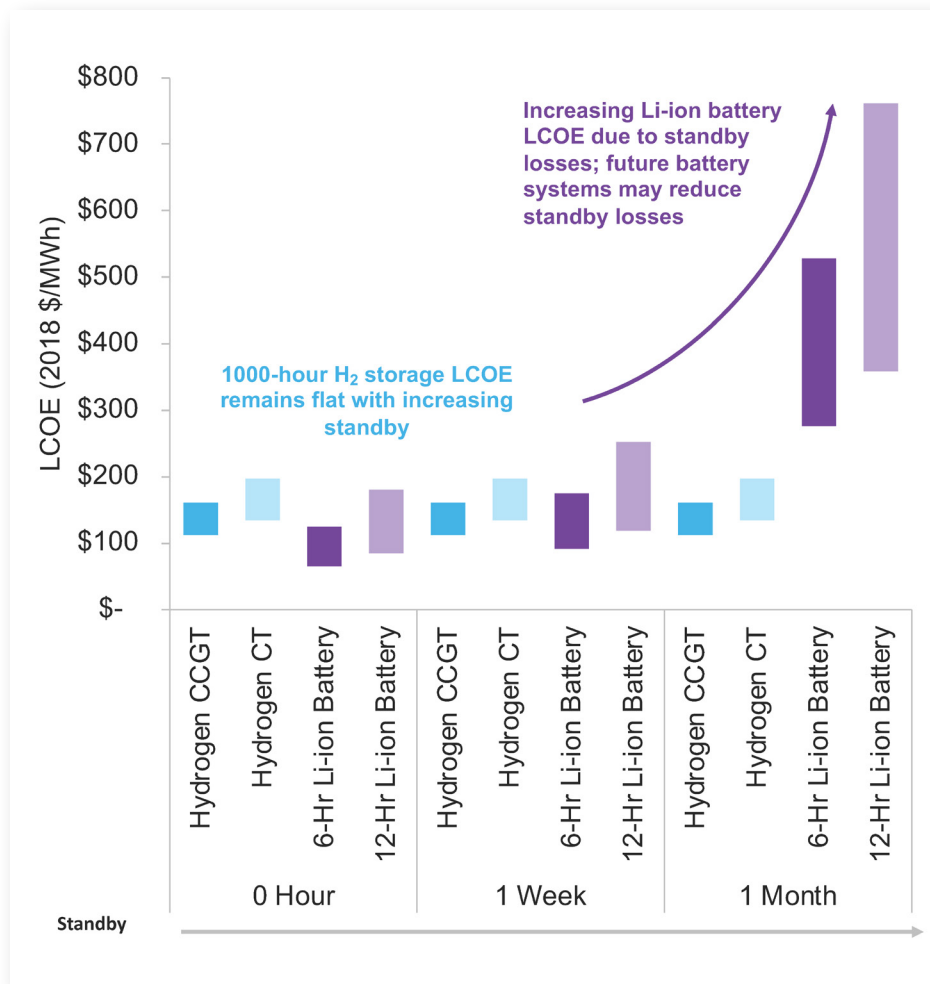
Figure 3-7: Comparison of LCOE between hydrogen storage and Li-ion battery storage at increasing standby durations, assuming Utah solar as a fuel and 2040 costs. 22
