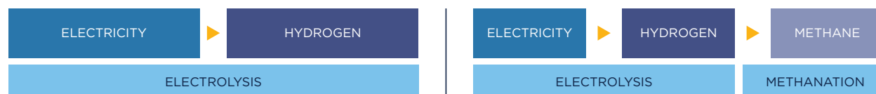
Figure 3: Power2Gas concepts: Power2Hydrogen and Power2Methane 53
